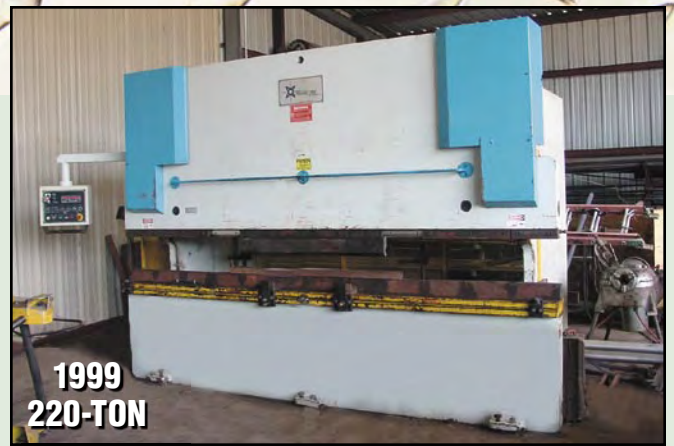
1999 220-TON PRIMELINE MDL. HAP37200 220-TON X 12' HYDRAULIC PRESS BRAKE
